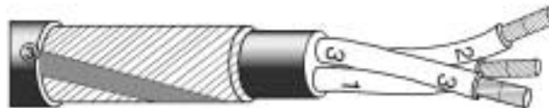
Figure 3-14 Concentric layer of copper wires with an open helix of copper tape.
