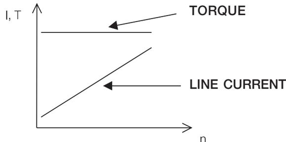
Figure 9.1 Line current in a constant torque application. Line current is small at low speed.
