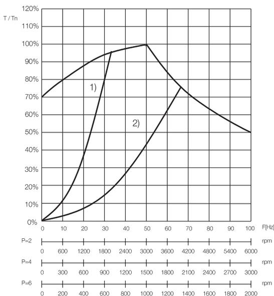
Figure 8.1 Motor loadability curves in a pump and fan application. Comparison of 1) 2-pole and 2) 4-pole motors.
