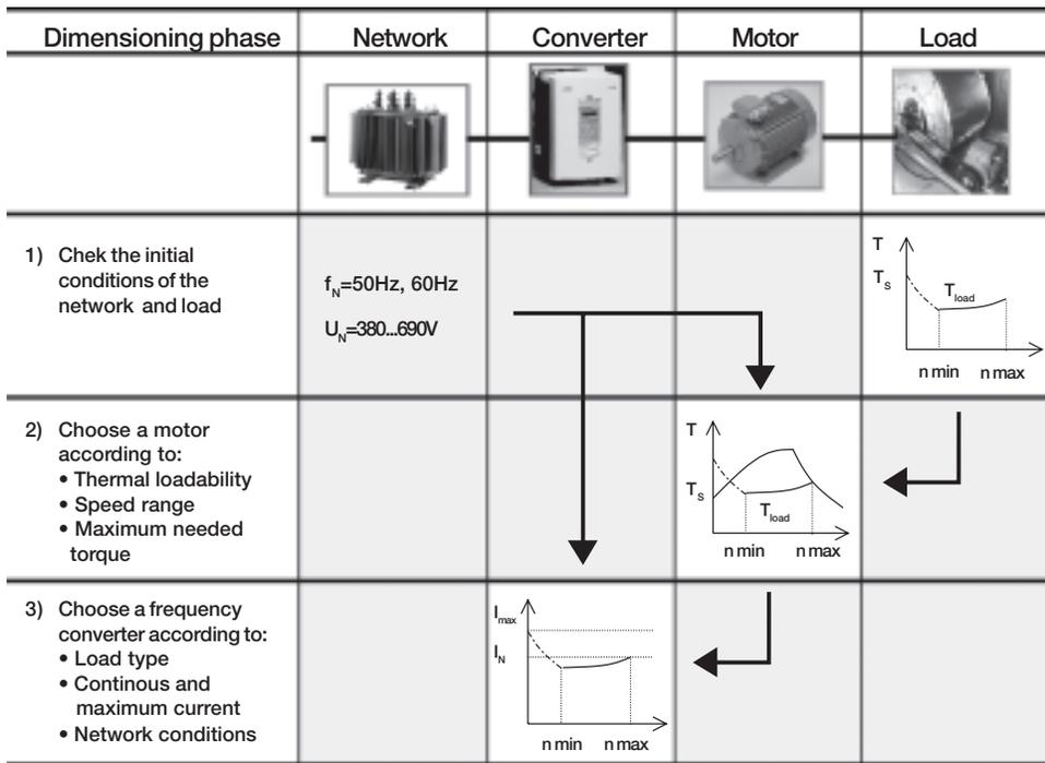
Figure 3.1 General description of the dimensioning procedure.
