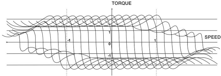
Figure 4.2 Torque/speed curves of an induction motor fed by a frequency converter.  $T_{max}$  is available for short term overloads below the field weakening point. Frequency converters, however, typically limit the maximum available torque to 70% of  $T_{max}$ .
