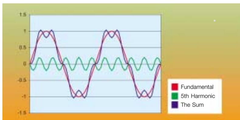
The distorted current or voltage waveform is the sum of the fundamental (e.g. 50 Hz) wave and harmonic (250 Hz in this example) wave.
